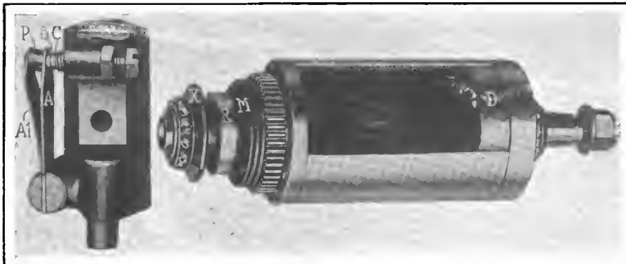
Fig. 2—Left—Detail of breaker mechanism. Right—Armature showing slip ring R and insulating rings M and X
